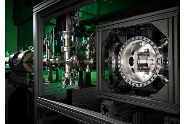
DICE facility, with right the molten salt chamber and beam target, and left the DIFFER accelerator
